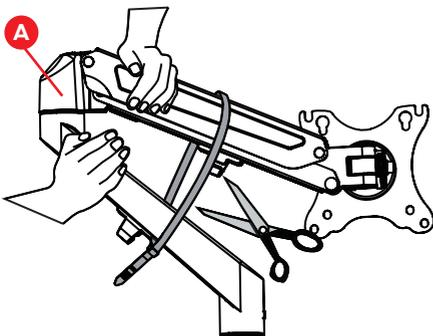
Firmly hold the 2 halves of the spring arm together and have another person cut off the cable tie from around the spring arm.
