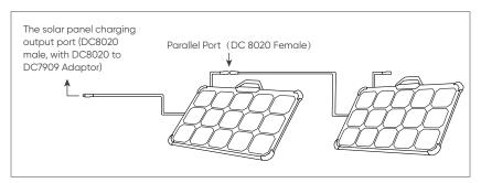
Tip: Users can enter the number of solar panels in their own combination according to the number of solar panels they purchased. Currently, the product supports charging with 1, 2, 3, 4, 6, 8, and 12 80W solar panels in combination.
