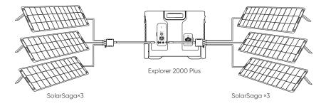
Caution: When the two inputs are used at the same time, please make sure to use the same type of solar panel and the number of solar panels in the two inputs must be the same to avoid damage or charging problems of the equipment due to inconsistent voltages of the two channels.
